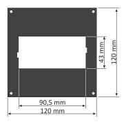
ITC-450/470 to mount 96 x 48 mm size unit in place of 96 x 96 mm cut-out
